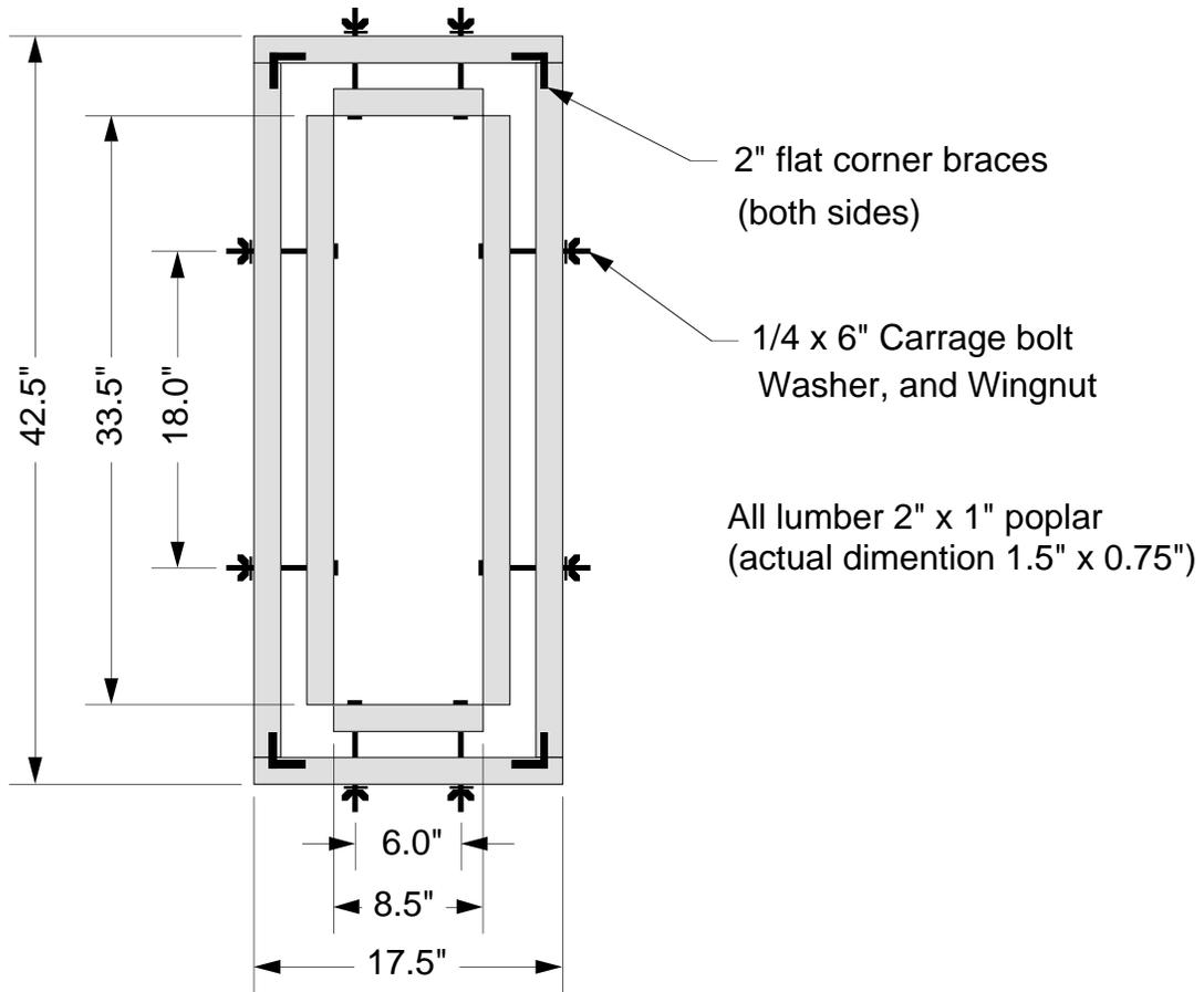
Mylar stretching Jig for Quad ESL tweeters.
