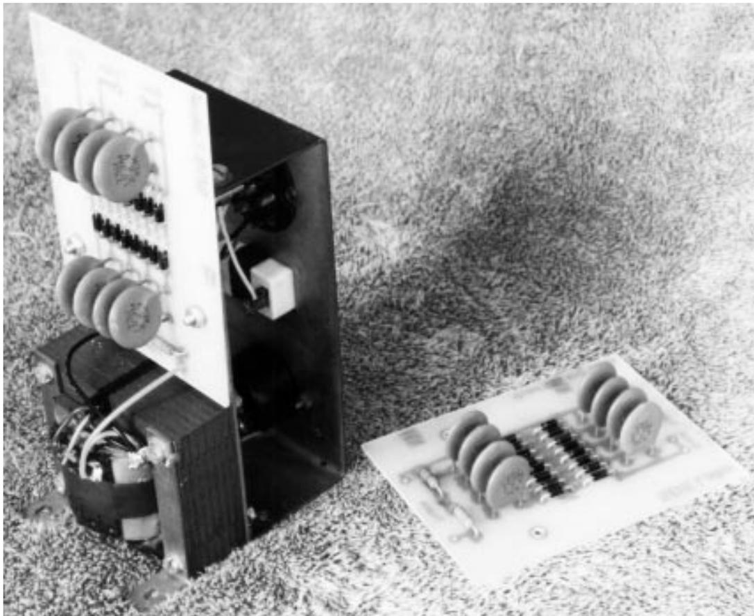
**Figure 5:** Quad ESL Power supplies (new circuit cards)
