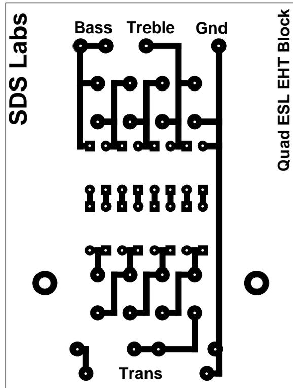
**Figure 6:** Replacement Rectifier Block Design
