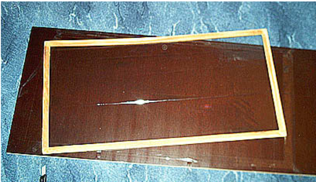
glueing the window-sealing-foil to the bass panels`s wooden dustcover-frames
